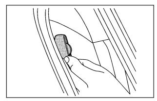
Slide the guide off of its storage clip located between the interior body and the seatback.
